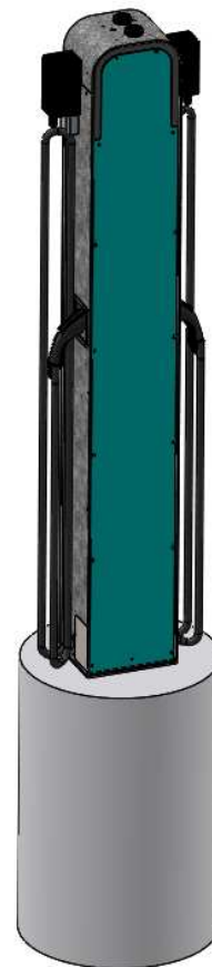
Minimum Pier dimensions: 24" diameter x 36" deep
